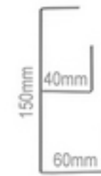
DCT 6 600mm wide x 60mm deep x 150mm high DCT 7 750mm wide x 60mm deep x 150mm high
